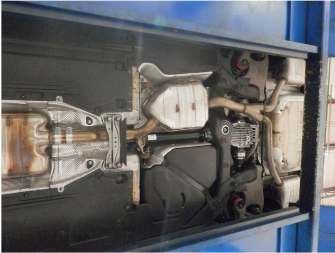
**Step 1.** To remove the OEM exhaust system you will first need to loosen the clamp assembly just behind the vehicles front resonator. Working front to rear disengage all hangers from the rubber insulators. The OEM system may now be removed in one piece. Retain all mounting hardware and rubber insulators as they will be needed to mount your new system.
