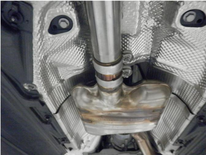
**Step 2.** Install your new MAGNAFLOW system by inserting the inlet end of the Inlet Pipe Assembly into the loosened OEM clamp. Locate the welded hangers to the rubber insulators. Keep all clamps loose for final adjustment of the system.
