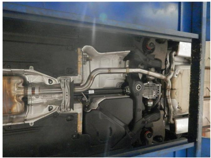
**Step 3.** Next loosely attach the inlet of the Y-Pipe Assembly to the outlet of the Inlet Pipe Assembly using the supplied clamp.
