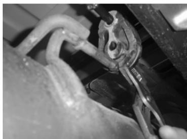
9. Remove muffler hangers from rubber isolators.
