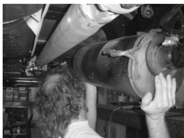
10. Remove factory muffler assembly.
