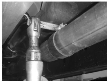
8. Using the 15mm socket and ratchet, loosen the clamp that secures the muffler assembly to the resonator/intermediate pipe.
