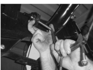
11. Install muffler hanger clamp into rubber isolators near the rear of the factory muffler location.
