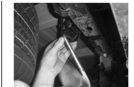
16. Insert tip and hanger into rubber isolator at the rear of the vehicle, near the spare tire.
