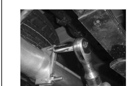
17. Position exhaust clamp over slip connection on tip. Repeat for Left side.
