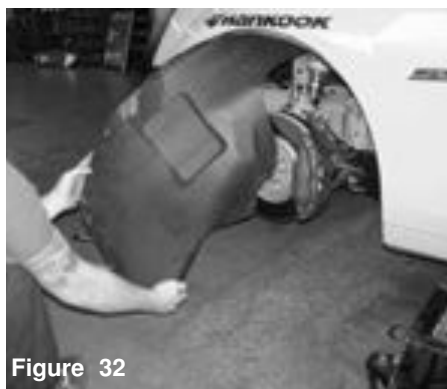
REAR VIEW- Here is another shot of the mud guard being pulled back.
