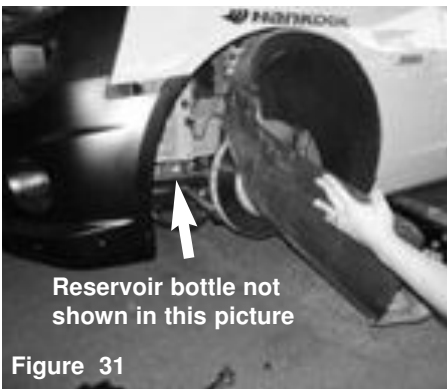
FRONT VIEW- Once you have removed the plastic clip, continue to pull the mud guard back.
