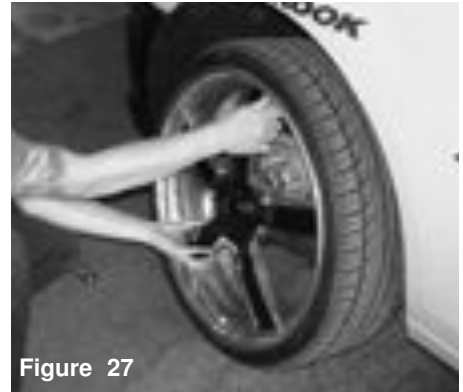
Once the car is lifted and safe to do so, continue to pull the wheel off. Note: When reinstalling the wheel be sure to torque lug nuts to factory specs.
