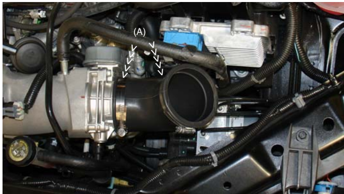
Prior to installing the elbow place a clamp over each end of the elbow (A). Take the 60 degree elbow and press the 2 7/8" over the throttle body. Position the 3" inlet side so that it faces upward.
