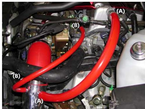
Take the 18" 17mm hose and press one end over the crank case port and the other end over the 3/4" port on the intake(A). The 20" 4mm hose has been connected to both ports (B).
