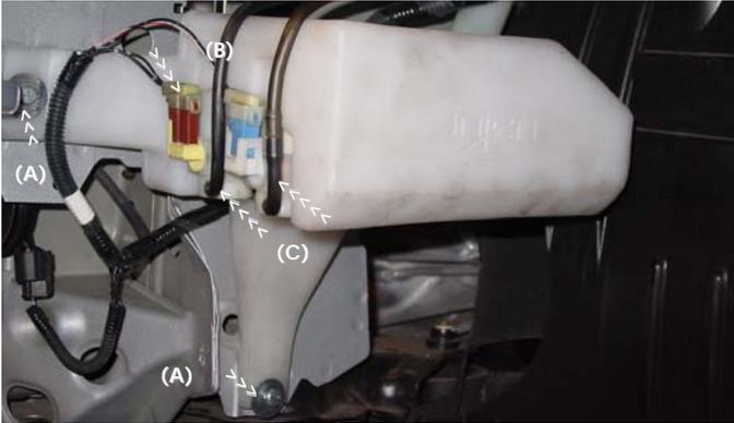
Use the m6 x m25 bolts and fender washers to secure the two extended legs on the reservoir tank (A). Plug the harness clips into the stock motors (B). Reconnect the stock rear and front lines to the original motors pumps (C).
