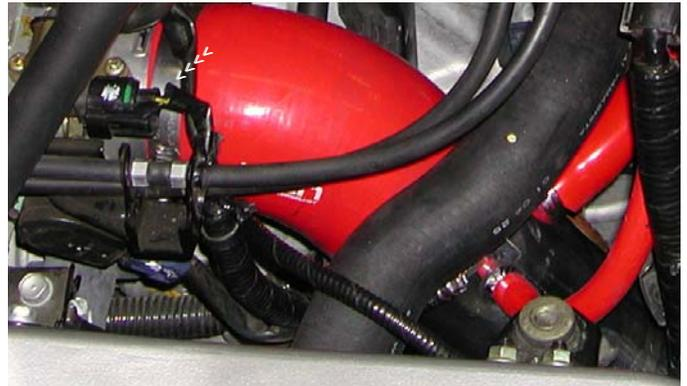
Press the 2 7/8" end of the molded elbow over the throttle body. Position the elbow downward and semi-tighten one of the clamps on the elbow.
