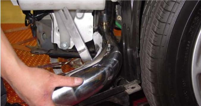
Insert the top end of the intake into the hole cut out made earlier, slip the intake up and into the engine compartment. Carefully insert the top end of the intake into the hose on the throttle body.
