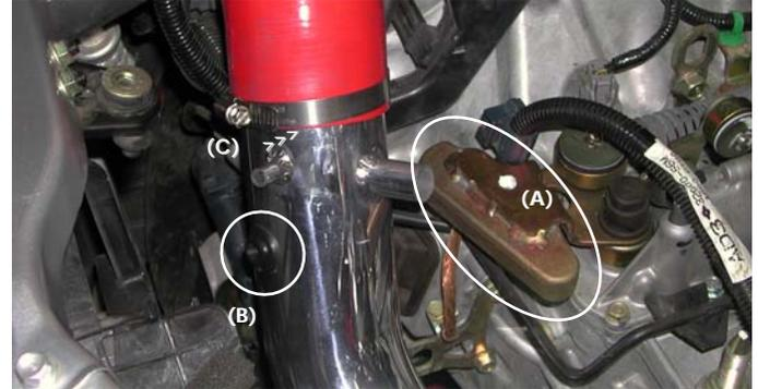
Set the transmission if 5th gear so that the lever is at its furthest point(A). Press the sensor grommet into the pre-drilled 3/4" hole on the intake (B). Align the intake for best possible fit so that nothing obstructs the intake, then continue to semi-tighten the clamp on the intake side (C).
