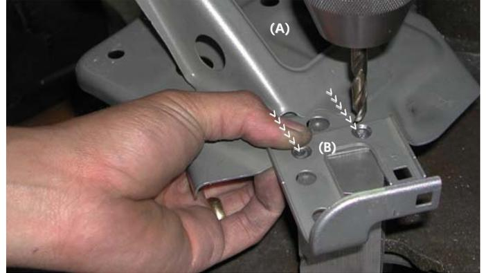
The battery tray is removed from the RSX (A). Turn the battery tray upside down and drill the two tacked or spot welded areas until the bracket becomes loose (B).
