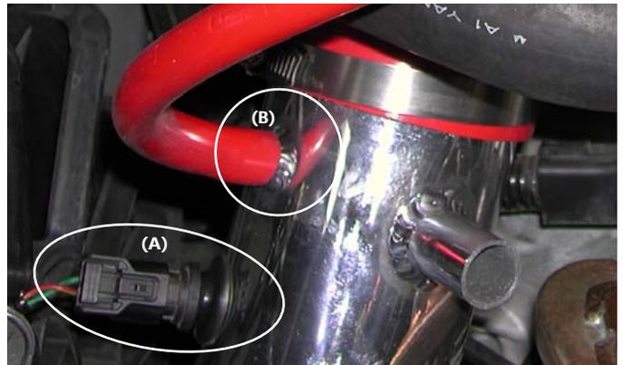
Take the air temperature sensor and press it into the grommet installed earlier (A). Take the 20" 4mm hose can press one end into the brake booster port and press the other end over the 3/8" port on the intake (B).
