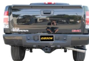
8. Install stainless steel tip #E. Clamp down. When you have everything in place, firmly tighten all bolts and clamps down securely. Use stainless steel or aluminum cleaner to polish tips. Inspect all fasteners after 25-50 miles of operation and re-tighten as necessary.
