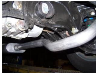
**4.** Install tailpipe and resonator assembly #C into muffler 1½"-2". Use clamp #E to secure to muffler. DO NOT TIGHTEN. Insert welded hangers into rubber grommets.
