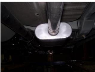
**3.** Install muffler #B onto head pipe 1½"-2" with the louvers facing towards the converter. Use a jack stand to support the muffler. Use clamp #E to secure the muffler to the headpipe. DO NOT TIGHTEN.
