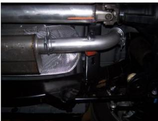
4. Install muffler #B onto head pipe #A 1 1/2"-2". Use a jack stand to support the muffler. DO NOT TIGHTEN. Muffler outlet is looking into the louvers.
