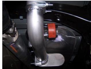
6. Install the intermediate tailpipe #C into the muffler 1 1/2"-2". Use clamp #G to secure tailpipe to muffler. DO NOT TIGHTEN.
