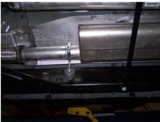
3. Install head pipe #A onto your existing stock flange and attach with factory hardware.
