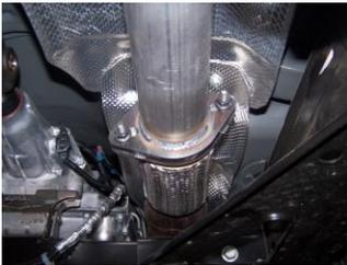
2. To remove the stock exhaust remove it from the flange located in front of your stock muffler. Disengage the welded hangers using WD-40 from the OEM rubber grommets. Do not damage or remove the rubber grommets as you will re-use them to mount your new system. Now, cut off tailpipe and remove exhaust.
