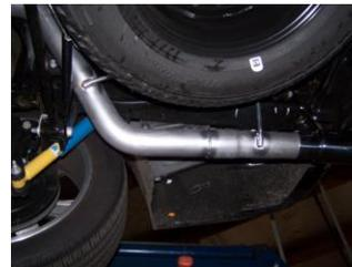
7. Install the overaxle tailpipe #D onto the intermediate tailpipe 1 1/2"-2". Use clamp #G to secure pipes together. DO NOT TIGHTEN. Insert welded hanger into rubber grommets.
