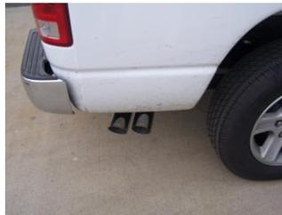
**6.** Install stainless steel tips. Clamp down. When you have everything in place, firmly tighten all bolts and clamps down securely. Use stainless steel cleaner and a Scotch Brite pad weekly to prevent tip from discoloration. Inspect all fasteners after 25-50 miles of operation and re-tighten as necessary
