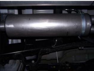
**3.** Install muffler #B onto head pipe #A 1 1/2"-2" with the louvers facing towards the converter. Use a jack stand to support the muffler. Use clamp #G to secure the muffler to the headpipe. Slide band clamp onto muffler and insert welded hangers into rubber grommets. Attach with bolt kit #J. DO NOT TIGHTEN. Muffler inlet is looking into the louvers.
