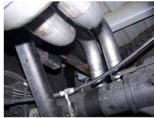
**4.** Install driver side tailpipe #C into muffler. Use clamp # F to secure. DO NOT TIGHTEN.
