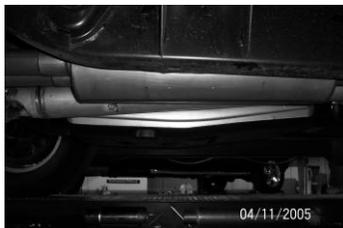
Install muffler #B onto head pipe 1-1/2" to 2" with the louvers facing towards the converter. Use a jack stand to support the muffler (make sure its level). Use clamp #G to secure the muffler to the head pipe. **Do not tighten.** Muffler inlet is looking into the louvers.
