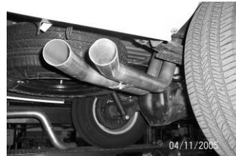
Install driver side over axle tailpipe # D into muffler and attach using clamp # F . Use bolt kit # H to attach the tailpipes together. **Do not tighten.** The driver side tailpipe tab will be on the bottom.
