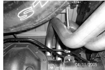
Install the passenger side over axle tailpipe # C into the muffler (1-1/2" to 2"). Use clamp # F to secure tailpipe to muffler. **Do not tighten.**
