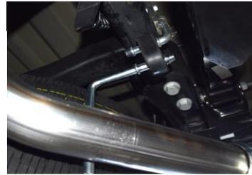
**6.** Install the driverside overaxle tailpipe #D into the muffler 1 1/2"-2". Use clamp #H to secure. **DO NOT TIGHTEN.** Rotate until it meets with the rubber grommet. **DO NOT TIGHTEN.**
