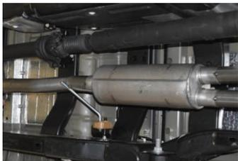
**3.** Install muffler #B onto head pipe #A 1 1/2"-2" with the louvers facing towards the converter and muffler outlets level. Use a jack stand to support the muffler. Use clamp #G to secure the muffler to the headpipe. Do not tighten. Muffler inlet is looking into the louvers.
