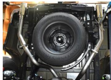
**7.** Next install the exit pipes #E. Use clamp #H to secure. **DO NOT TIGHTEN.** Rotate pipes to your desired look.
