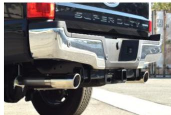
**8.** Install stainless steel tips. Clamp down. When you have everything in place, firmly tighten all bolts and clamps down securely. Use stainless steel cleaner weekly to prevent tip from discoloration. Inspect all fasteners after 25-50 miles of operation and re-tighten as necessary
