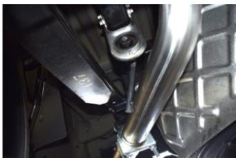
**4.** Install the passenger side overaxle tailpipe #C into the muffler 1 1/2"-2". Use clamp #H to secure tailpipe to muffler. **DO NOT TIGHTEN.** Insert hangers into rubber grommets.
