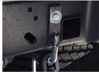
**5.** Install hanger #I into hole that is already threaded to receive the bolt Item# J on the driverside frame rail just rear of the axle. You will use the lower right side bolt hole. There will be 4 choices in the correct area. **DO NOT TIGHTEN.** Install rubber grommet
