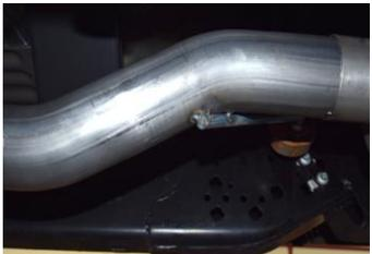
**2.** Install head pipe #A onto your existing stock front pipe and attach with clamp #G. Insert welded hanger into rubber grommet.
