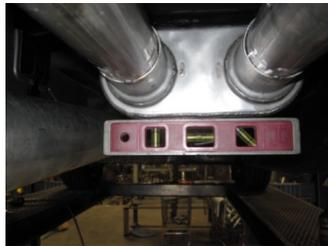
4. Install muffler #B with inlet stands to support the muffler. Use clamp #F to secure the muffler to headpipe. Do not tighten.
