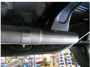
2) If installing the system on a Crew Cab truck with a 6.5' bed, place extension pipe **#TB700S** onto the back of the **#26401S** inlet pipe, place a provided clamp onto the slip-fit and tighten enough to hold in position. This extension pipe will not be used on Double Cab or Crew Cab-5.5' bed models.
