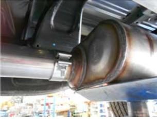
3) Place a supplied 3" clamp over the inlet of the muffler, then slide the inlet of muffler onto the back of the inlet pipe. Use a stand to support the muffler. Tighten the clamp just enough to hold in position.
