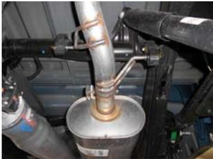
2) Support the muffer with a stand. Using a hacksaw or sawsall, cut the stock tailpipe off just behind the muffer. Separate the wire hangers on the tailpipe from the rubber mounts on the vehicle and remove the tailpipe from the vehicle. This step is not mandatory but makes removal easier.
