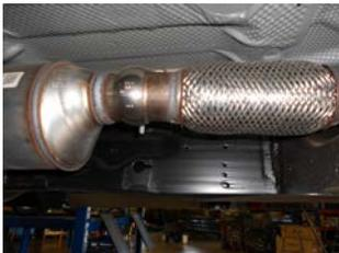
3) Using a 15mm wrench, loosen the bolt on the clamped ball connection behind the catalytic converter. Separate the wire hangers from the rubber mounts on the vehicle and lower the inlet pipe and muffer from the vehicle. A lubricant will make removal much easier. You will need to remove the ball clamp from the stock system; it will be reused with the Flowmaster system.
