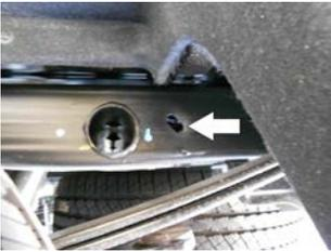
4) Slide rubber hanger **#HA168** onto the end of **226HA**, then using the supplied bolts, washers, nuts and backing plates **#HA566**, mount the assembly to the frame on the left side of the vehicle using the angled oblong hole on the frame rail. *Note: the backing plates #HA566 go on both sides of the frame between the hanger, washers & bolts to cover the oblong holes so that the frame hangers won't bend into the oblong holes.*
