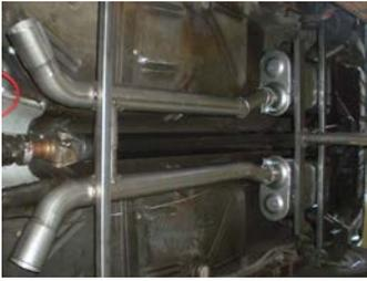
4) Install the front pipe assembly **#86189S** by placing the rear of the front pipe assembly into the inlets of both mufflers and centering it in the drive line cavity. (Be sure to install the clamps first.) Support the front of the assembly with a stand, and position the mufflers and front pipe assembly so that they are level. Once the mufflers and front pipe assembly are in place, check the tailpipe clearance where they go up in front of the rear axle to be sure there is adequate clearance.
