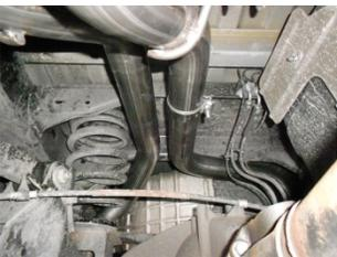
10) Connect the rear section of the left side tailpipe **#26467S** onto the back of the front section by sliding the two sections together at the slip-fit connection over the rear axle. Place the hanger at the rear of the tailpipe into the rubber mount installed in Step 7 above. Tighten the clamp enough to hold, but still allow for adjustment.
