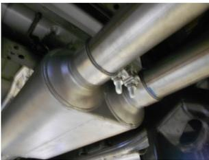
8) Install a provided 3" clamp onto the right muffler outlet. Place the right side tailpipe **#26465S** into position over the axle and slip into the right side muffler outlet, while at the same time, connecting the hangers at the front and rear of the pipe to the rubber mounts on the vehicle. Tighten the clamp enough to hold, but still allow for adjustment.
