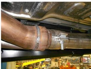
4) Place a provided 3 ½" clamp over the expanded end of inlet pipe **#36061S**, then place onto the stock front pipe just behind the catalytic converter. Be sure to line up the notch in the pipe with the tab on the front pipe. Connect the hanger on the pipe to the rubber mount on the vehicle and tighten the clamp enough to hold but still allow for adjustment.
