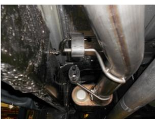
5) For Crew Cab - 6'-4" bed models place a provided 3 ½" clamp onto the expanded end of extension pipe **36062S**, place onto the back of the inlet pipe and connect the hanger on the pipe to the rubber mount on the vehicle. Tighten the clamp enough to hold but still allow for adjustment.
