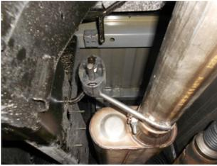
6) For Crew Cab - 8' bed models place a provided 3 1/2" clamp onto the expanded end of extension pipe **#36063S**, place onto the back of the inlet pipe and connect the hangers on the pipe to the rubber mounts on the vehicle. Place a provided clamp onto the muffler inlet, slide the muffler onto the back of the extension pipe and support the muffler with a stand. Tighten the clamp enough to hold but still allow for adjustment.
