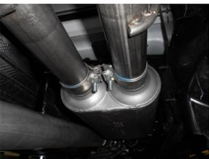
9) Install a provided 3" clamp onto the left muffler outlet. Place the front section of the left side tailpipe **#26466S** into the left side muffler outlet and connect the hanger on the pipe to the rubber mount on the vehicle. Tighten the clamp enough to hold, but still allow for adjustment. Place a second 3" onto the back of this pipe in preparation for the next step.
