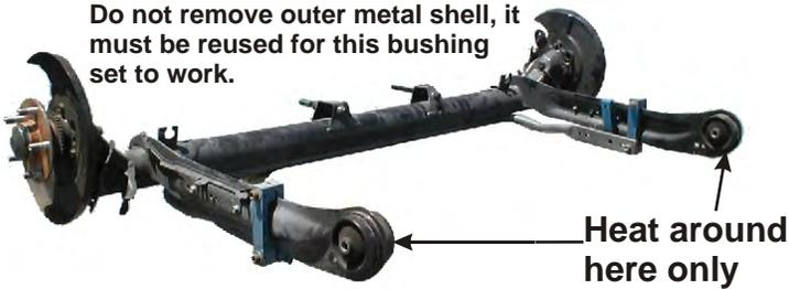
To remove rubber bushing, apply light heat evenly around the outside of the outer metal shell, just enough to break the bond with the rubber. When you see light smoke coming from the sides of the bushing the bond should be broken. (At no time should there be any flames coming from the rubber, if there are any flames, you need to back off with the heat). Just push the old rubber and inner metal sleeve out. Let the outer metal shell cool off before cleaning the
