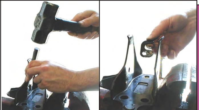
Use a chisel on the inside to break away remainder of tab. Use a file to remove all sharp edges that might cut or rip the new polyurethane bushings.
