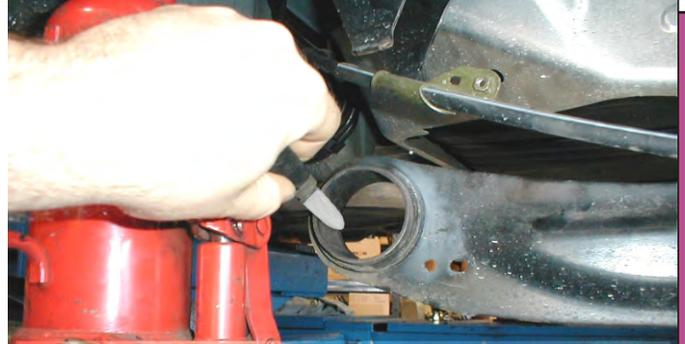
Let metal shell cool before cleaning inside. Remove any burrs and sharp edges before applying grease. With both eyes of the trailing arm smooth, clean, and free from sharp metal burrs and any metal shavings.
