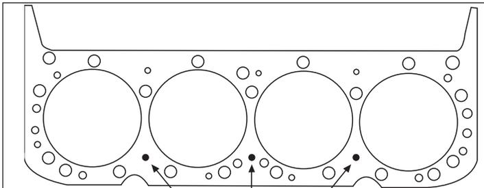
Drill three .125" holes in each head using 400 c.i.d. head gasket as a guide. **DRILL ONLY THE THREE LOWER STEAM HOLES** (closest to the spark plugs) as indicated. Drill straight into the head (90° from the deck) until the drill breaks through into the water jacket (about 9/16").
