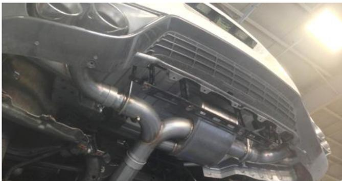
2. Visually inspect the tip alignment and clamp orientation. Make any necessary adjustments at the slip joints and flange connections.
