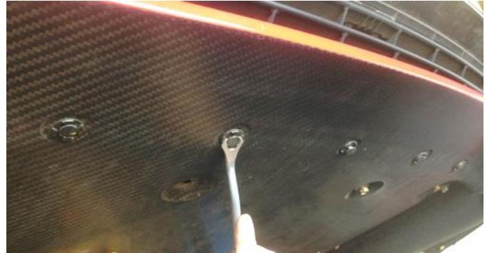
**1.** Remove the 11 plastic clips on the center and side under paneling with a clip removal tool.
