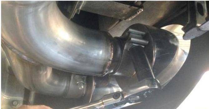
1. Hold the CORSA 5.0" tip with the logo facing up and slide a provided 65mm clamp onto the inlet so the hardware is to the inside of the vehicle, and the nut is downwards.
