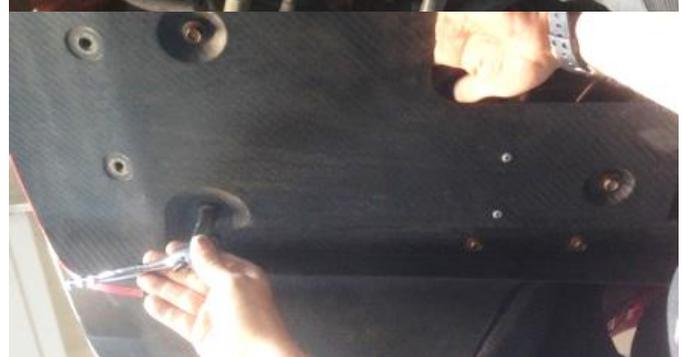
**2.** Remove the 15 larger sized bolts on the center under tray using a 12mm socket and ratchet.
