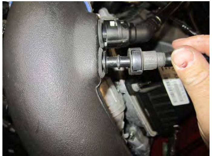
16. Press the factory breather lines onto the CORSA snap fittings.
