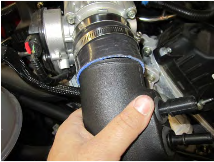
13. Slide the CORSA duct into the 3in sleeve, do not tighten the clamp at this time.
