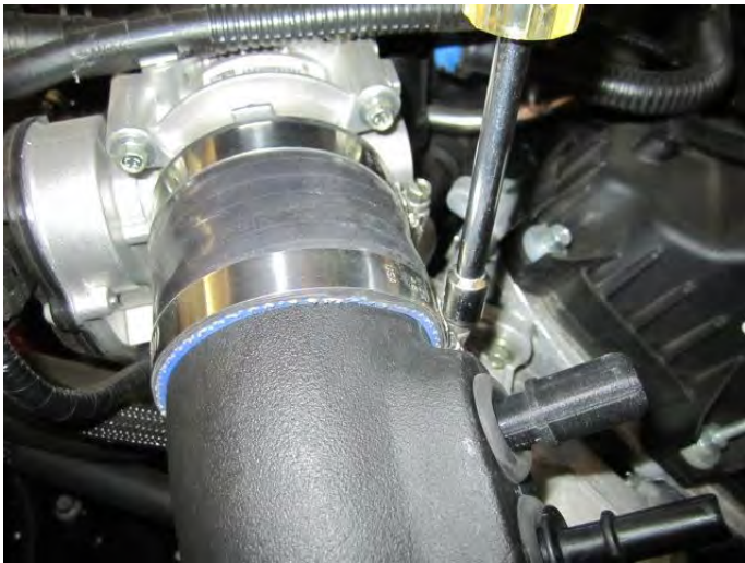
15. Tighten the clamp holding the duct to the 3in sleeve using a 5/16 socket or nut driver only.
