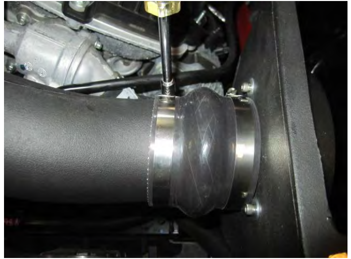
14. Tighten the clamp holding the duct to the hump hose using a 5/16 socket or nut driver only.
