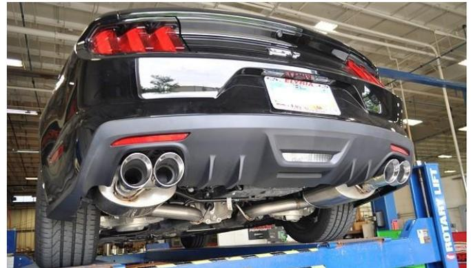
**3.** Adjust the position and depth of the tip assemblies until it is centered in the cutout, and has an equal amount of reveal on each side, then tighten the clamps using a 15mm socket and 3/8" ratchet. Torque the clamps to 45ft-lb using a torque wrench and 15mm socket, ensuring that the tips are still in the desired position.
