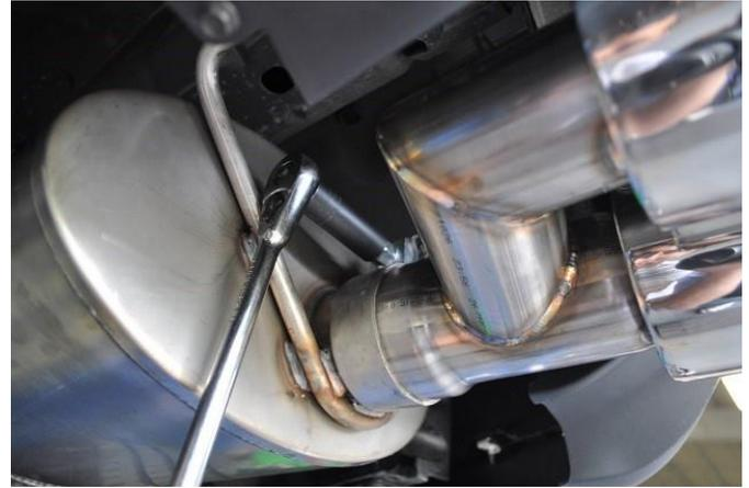
**1. CAREFULLY** insert the tip assembly into the driver side muffler outlet pipe and snug the clamp using a 15mm socket, 3/8" driver ratchet and 3" extension.
