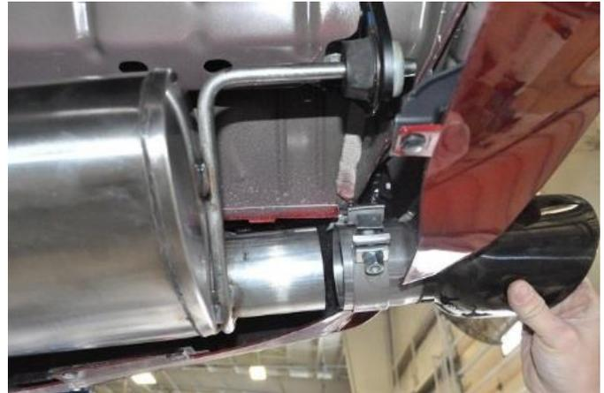
**2.** CAREFULLY remove the tip assembly from the mufflers to free it from the vehicle.
