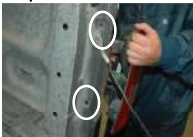
Remove the passenger side tail light by removing the two 8mm
