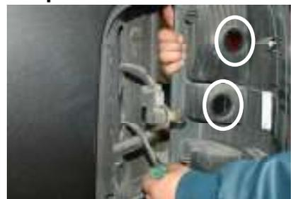
Remove the reverse and the brake light bulbs from its sockets.
