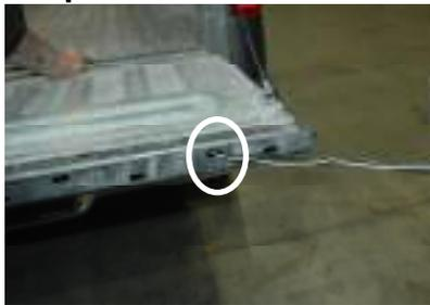
Slide the part of Anzo Spoiler wire loom connected to the Spoiler through the opening within the top of the tail gate.
