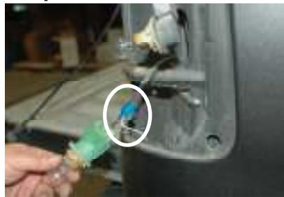
Splice the white Anzo Spoiler power source wire to the red reverse light power source wire.
