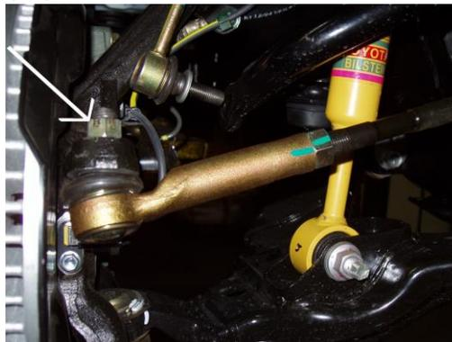
8. Screw the tie rod end nut upside down (the safety pin slots facing the ground) back on to the tie rod end bolt until the top of the bolt is level with the top of the nut. Make sure the threads of the bolt are not higher than the nut. Using a hammer hit the tie rod end bolt out of its place. Once the tie rod end bolt breaks loose remove the nut and the tie rod end.
