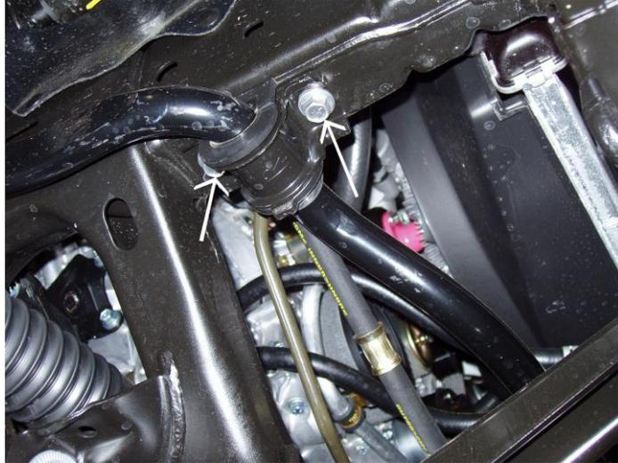
12. Using a **14mm** wrench or socket remove the three nuts from the top of the OEM spring hat.
