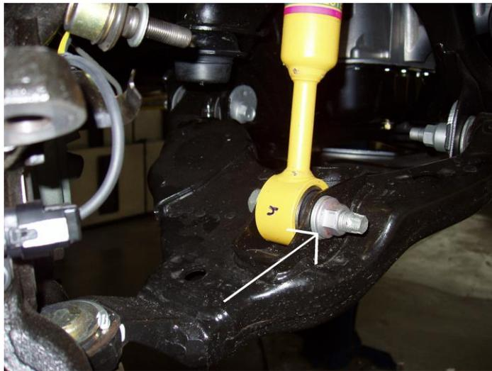
14. To install your new *Sway-A-Way* shocks align the upper shock mount inside the stock coil housing with the hose fitting facing outwards and hoses pointing towards the front of the truck. Loosely secure with the supplied 3/8" bolts and lock washers.
